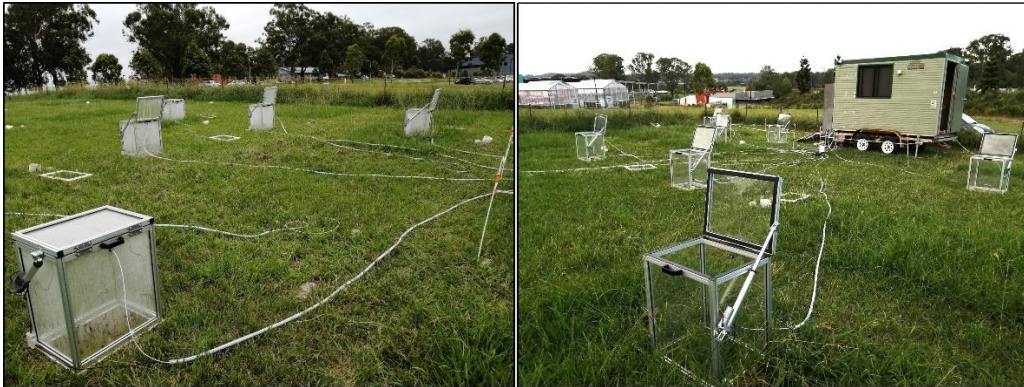
Fig. S1. Chamber system installed on-site for GHG measurements.
