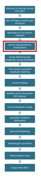
Survey Regularisation and Interpolation Common grid – orientated to structure
