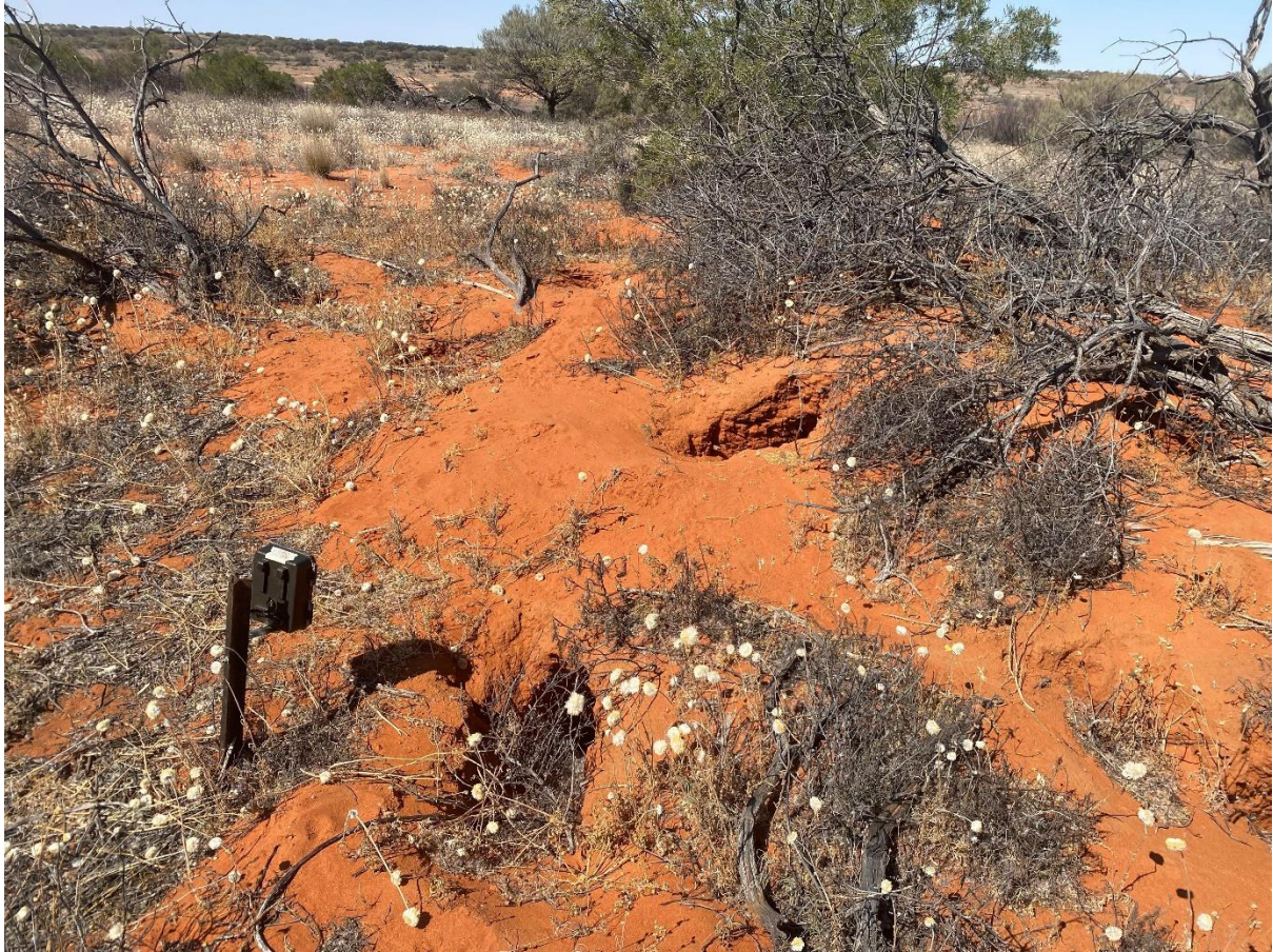
Fig. S2 Camera trap layout at a woma shelter-site. Swift Enduro trail cameras were positioned within 1 m of the largest burrow and were aimed down at angle of 60°, producing a 1 m 2 field of view (credit: Josh Magro).
