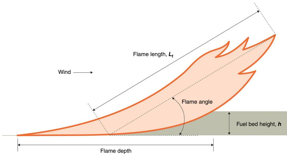
**Fig. 1.** Schematic representation of the cross-section of a wind-driven fire head showing flame length ( $L_f$ ) as considered in the present study, i.e. assessed along its axis from the tip of the flame to the base of the fuel bed.
