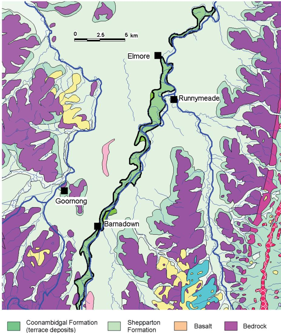
Fig. 16. Geology of the Campaspe Plains with the Coonambidgal Formation strip aquifer along which the Campaspe River flows.
