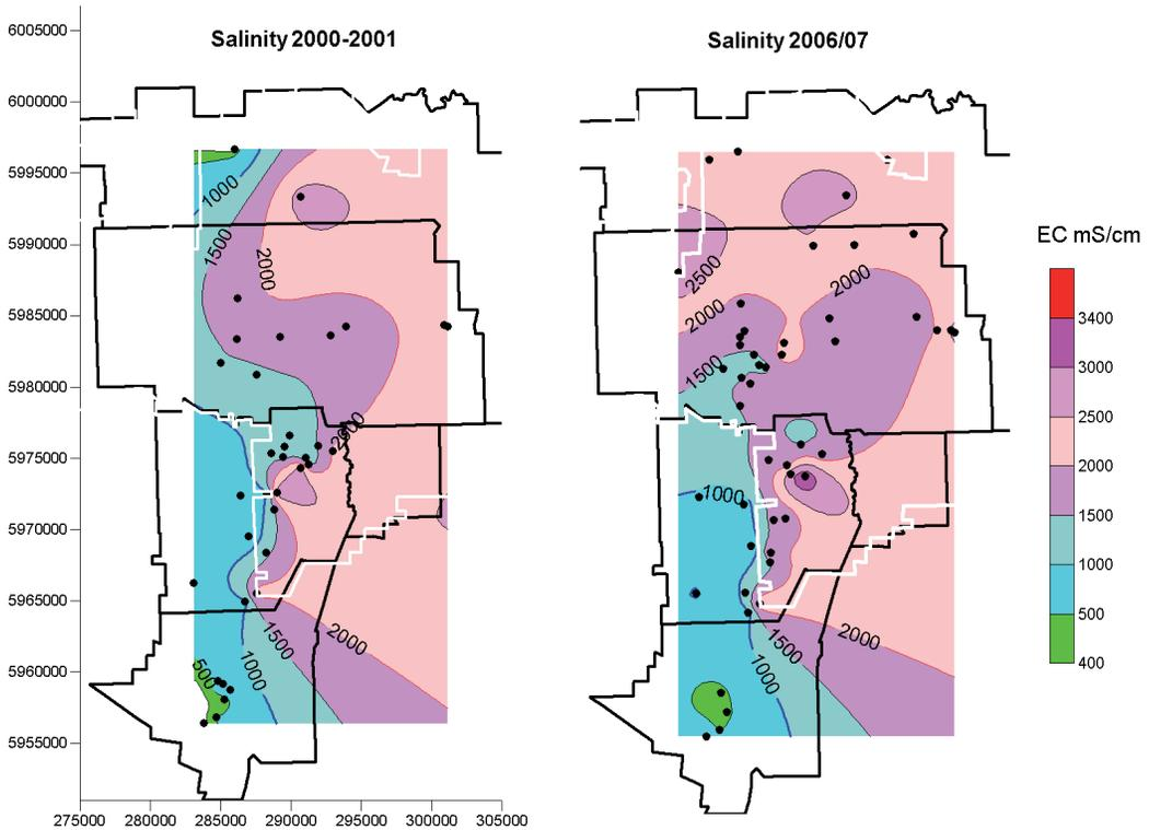
Fig. 36. Groundwater salinity of the Calivil/Renmark aquifer in 2000/2001 and 2006/2007 in the central-lower Campaspe Valley.
