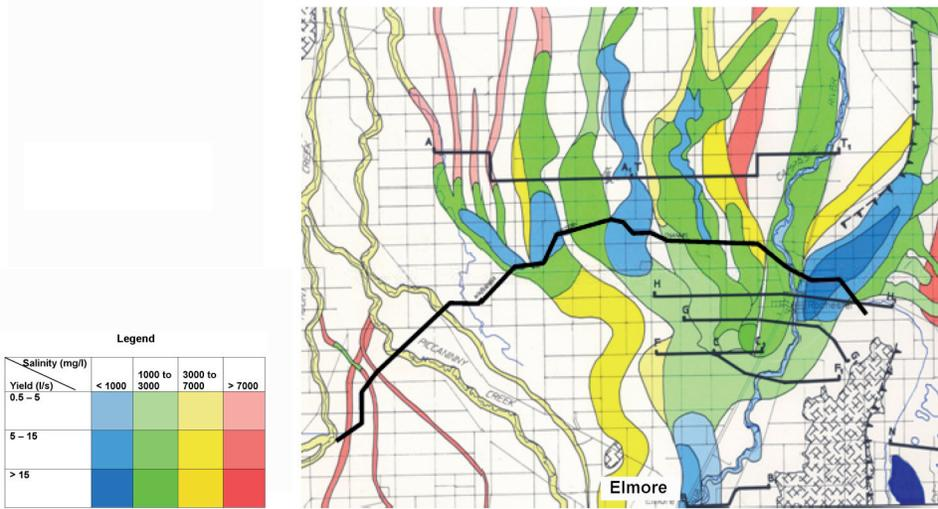
Fig. 22. Hydrogeological map of the area north of Elmore showing the salinity of shallow Shepparton Formation prior-stream aquifers. Fresh water plumes of recharged groundwater commence in the vicinity of the Campaspe River near Elmore, and in the vicinity of the Waranga Channel (from Ife 1988).
