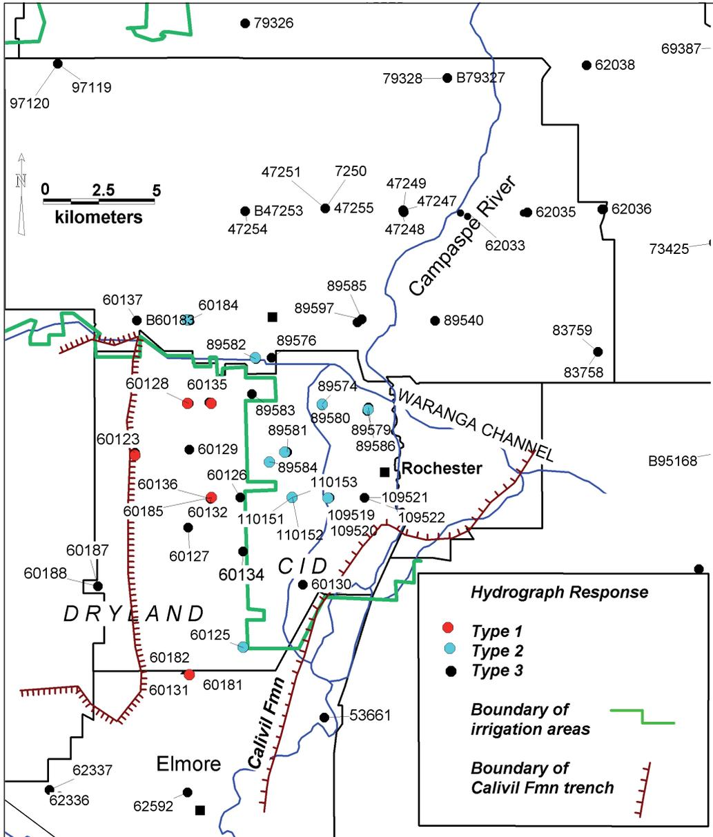
Fig. 34. Distribution of hydrograph types in the central-lower Campaspe Valley.
