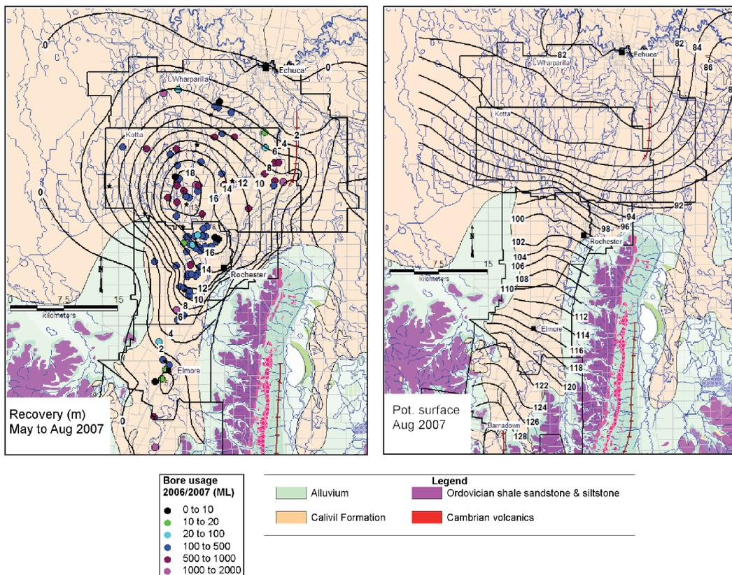
Fig. 30. Potentiometric surface of Calivil Formation August 2007 and extent of recovery from May 2007.
