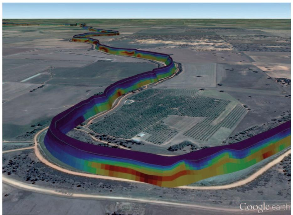
**Figure 3.** Electrical resistivity projected along a canal. The aqua line represents the canal bed. Reds in the sections are conductive, while purples are resistive. Indurated bedrock, weathered eluvium, and possibly windblown sand, are inferred to be representative of the materials under this canal.
