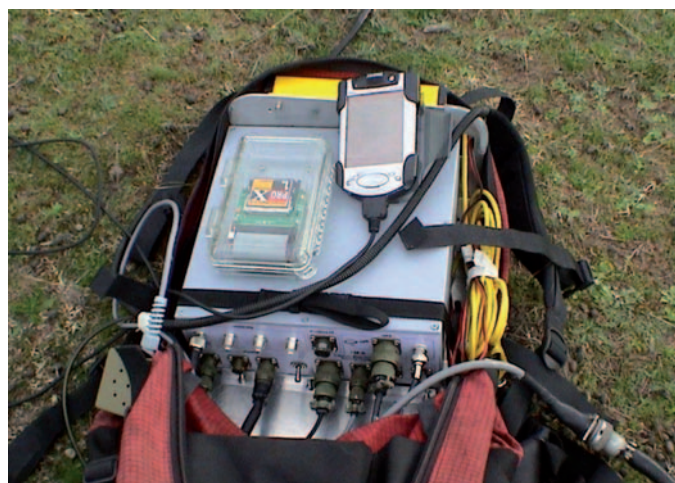
Figure 8. The TM-6 magnetometer system with ports for up to four Cs sensors and a frequency counter capable of delivering measurements to 0.04 nT resolution 2400 times per second with each measurement time tagged to 10 \mu s precision synchronised to GPS time. Data positioning with cm accuracy and survey navigation aids was provided by DGPS. On-board signal stacking delivered a noise floor of just 0.05 pT for electromagnetic exploration applications.
