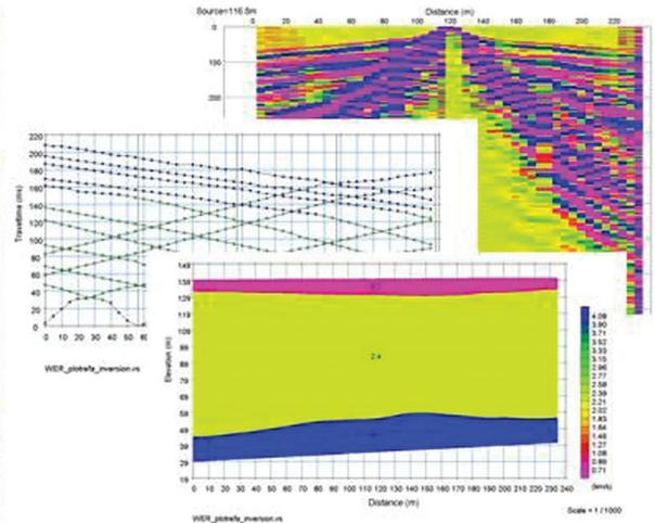
**Figure 3.** Basement depth estimates from 2015 ground geophysical survey results will be tested by drilling. An ‘explorer’s toolbox’ is being developed for the Southern Thomson region.
