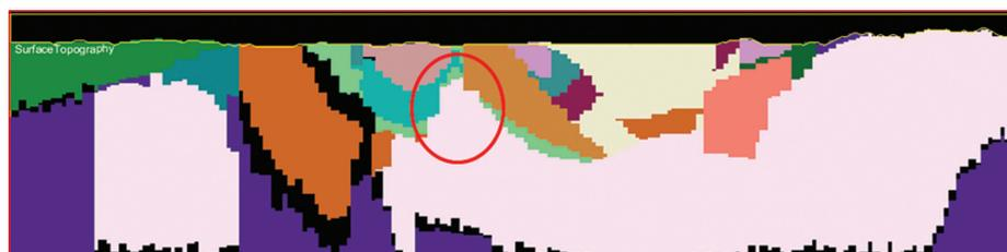
**Figure 8.** East-west 'probability threshold' section through TCGA (red ellipse), showing presence of units in >90% of acceptable solutions.
