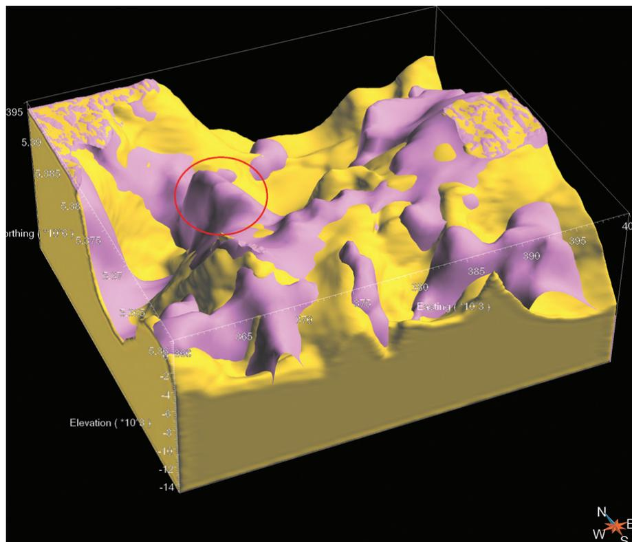
**Figure 7.** Granite surfaces in the northern part of the model before (yellow) and after (pink) the 3D gravity geometry inversion phase.
