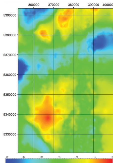
**Figure 6.** Bouguer gravity (terrain-corrected, mGal).
