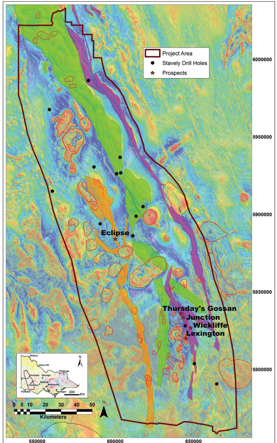
**Figure 1.** Stavely Project area showing Stavely Arc volcanic belts as coloured screens, Cambrian and Devonian intrusions with red outlines, stratigraphic drill hole collar locations and mineral prospects on a tilt-filtered TMI image.
