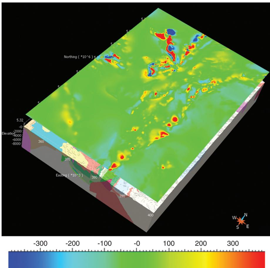
**Figure 4.** Residual magnetic intensity (observed – model) following homogeneous inversion (nT).
