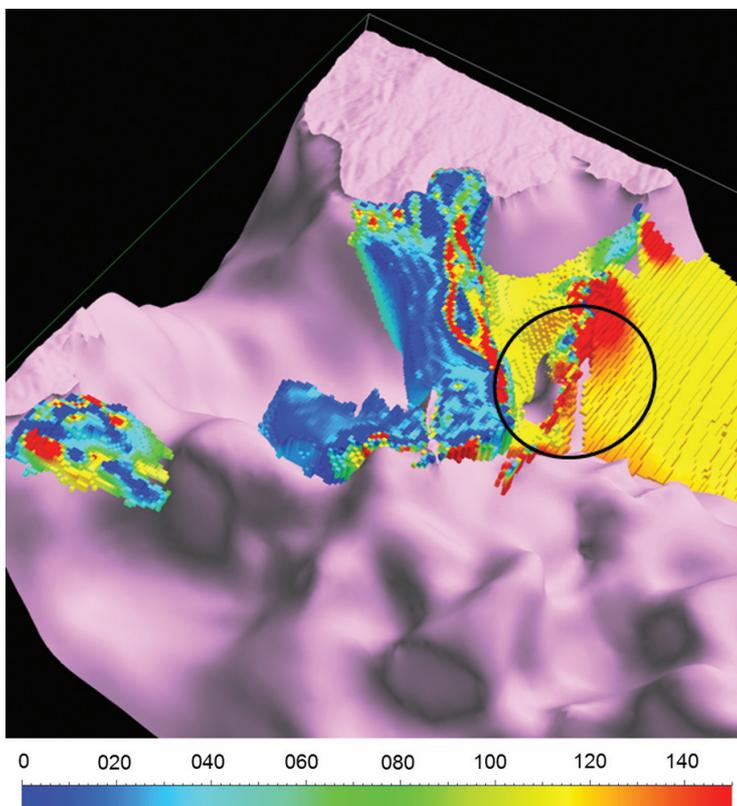
**Figure 5.** Apparent magnetic susceptibility ( $SI \times 10^{-3}$ ) within Crimson Creek Formation and ultramafic complexes, resulting from heterogeneous inversion.
