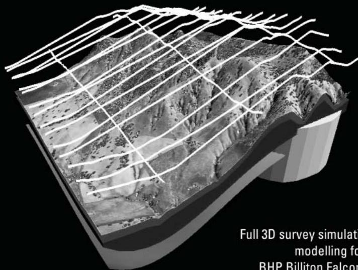
Full 3D survey simulation & modelling for the BHP Billiton Falcon and Bell Geospace airborne gravity gradiometer systems
