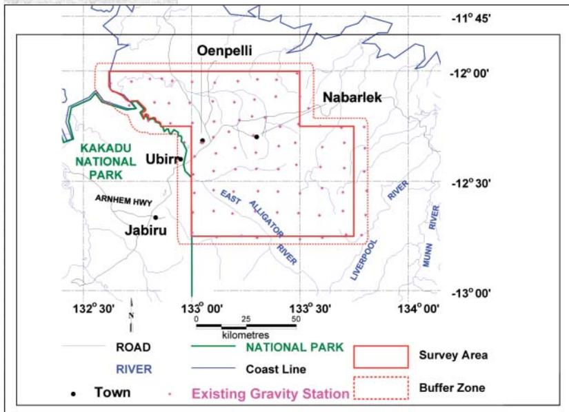
Fig. 1. Location of the West Arnhem Land airborne geophysical survey.
