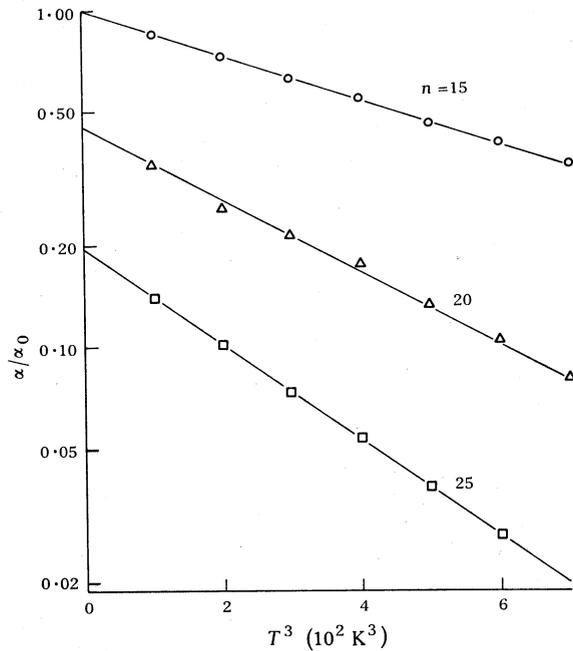
Fig. 2. Reduced attenuation  $\alpha/\alpha_0$  versus  $T^3$  for longitudinal wave magnetoacoustic data at 152 MHz with  $\mathbf{q}$  along [011] and  $\mathbf{H}$  along [100]. Plots are shown for harmonic numbers  $n = 15, 20$  and  $25$  (the latter two plots being displaced vertically for clarity).
