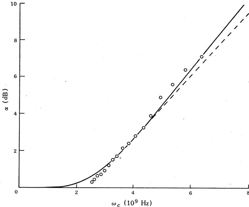
Fig. 4. Fit of the data corresponding to Fig. 1 to equation (1) (full curve) and equation (3) (dashed curve) for a total scattering rate  $\nu = 3.25 \times 10^9 \text{ s}^{-1}$ .
