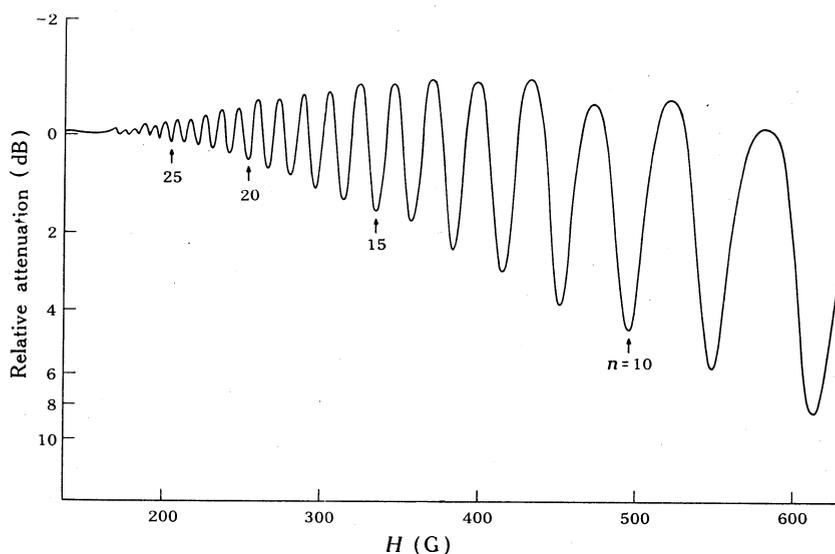
Fig. 1. Typical magnetoacoustic oscillations for 152 MHz longitudinal waves propagating along [011] in high purity copper. The temperature was 4.65 K and the field  $H$  was along [100]. Note the decrease in amplitude with increasing harmonic number  $n$ . (Note also  $1 \text{ G} \equiv 10^{-4} \text{ T}$ .)
