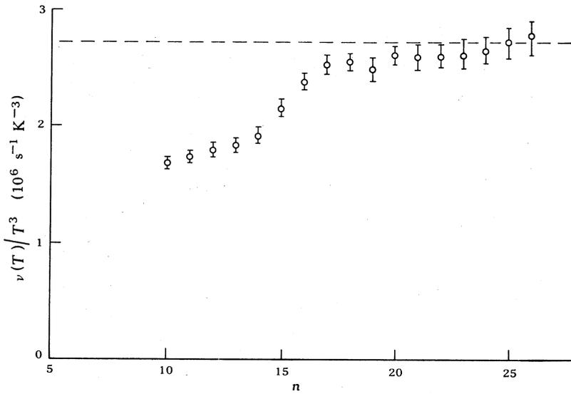
Fig. 3. Plot of the coefficient  $a = \nu(T)/T^3$  as a function of harmonic number  $n$  for the data corresponding to Fig. 2. The dashed line gives the corrected value obtained from RFSE data for this field orientation.
