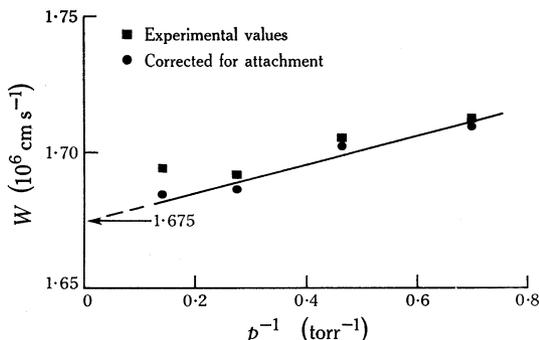
Fig. 3.—Variation of the measured drift velocity  $W$  with  $p^{-1}$  at  $E/N = 1.81$  Td. The experimental results have been corrected for attachment by the method described in Section IV and the value of  $W$  then found by linear extrapolation.
