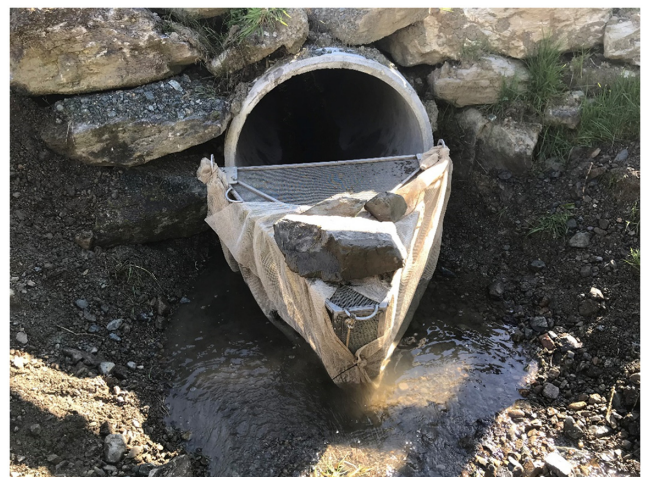
Fig. 2. Whitebait trap installed at the culvert inlet to capture fish successfully passing the structure.
