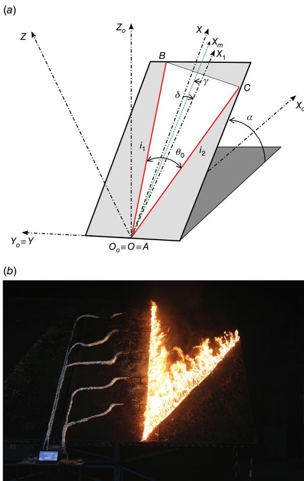
**Fig. 1.** (a) Schematic layout of the merging of two non-symmetric straight fire lines making an initial angle  $\theta_0$  between them. The axis  $OX$  is parallel to the slope gradient, the axis  $OX_1$  represents the symmetry line of the fire configuration and the axis  $OX_m$ , defined by the green dashed line, represents the maximum ROS. (b) View of the Canyon Table DE4 of the Forest Fire Laboratory of the University of Coimbra.
