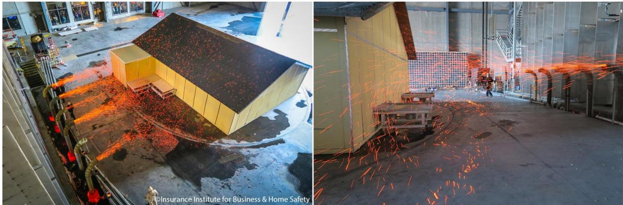
**Fig. 4.** Test building and ember generator system used in the accumulation study. As shown, (left) the collection trays were initially covered with a solid panel until steady flow from the generators was observed, at which point the covers were removed (right) allowing embers to land in the water-filled pans.
