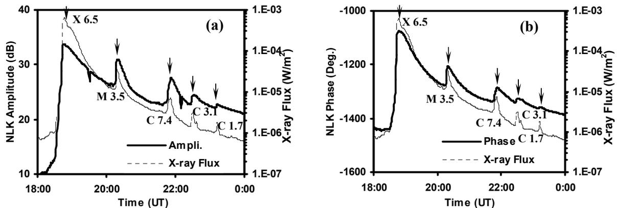
**Figure 2 (a, b)** Variation in the amplitude (a) and phase (b) of NLK signal along with the GOES X-ray flux during the solar flares on 6 December 2006.
