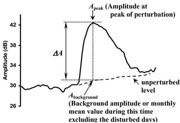
**Figure 1** Method of determining the perturbation (enhancement) in the amplitude of VLF signals during the solar flares.
