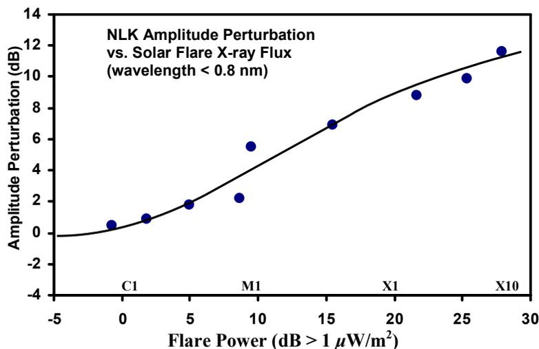
**Figure 3** Solar flare induced amplitude enhancement in NLK signal as function of peak solar flare X-ray flux in dB (relative to 1 μW/m<sup>2</sup>) in the 0.1-0.8 nm band.
