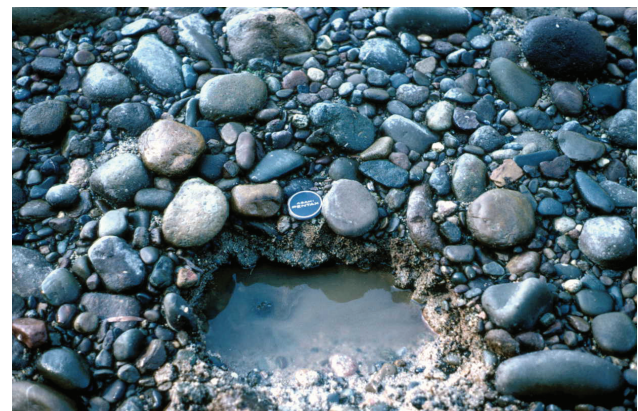
Figure 7: Moderately well sorted, fine skewed, mesokurtic, pebble gravel armour layer overlying low bearing strength very poorly sorted, coarse skewed, very platykurtic, sandy pebble gravel sub-armour sediment on longitudinal bar at cross section 8 at Sandy Point. See Figure 3 for location of cross section.
