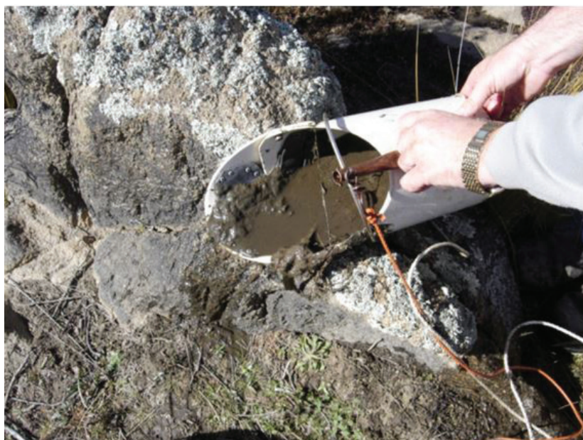
Figure 6: The scoop bed sediment sampler in use at a benchmarking site in the Dalgety Uplands Reach. For location of river reach, see Figure 1.
