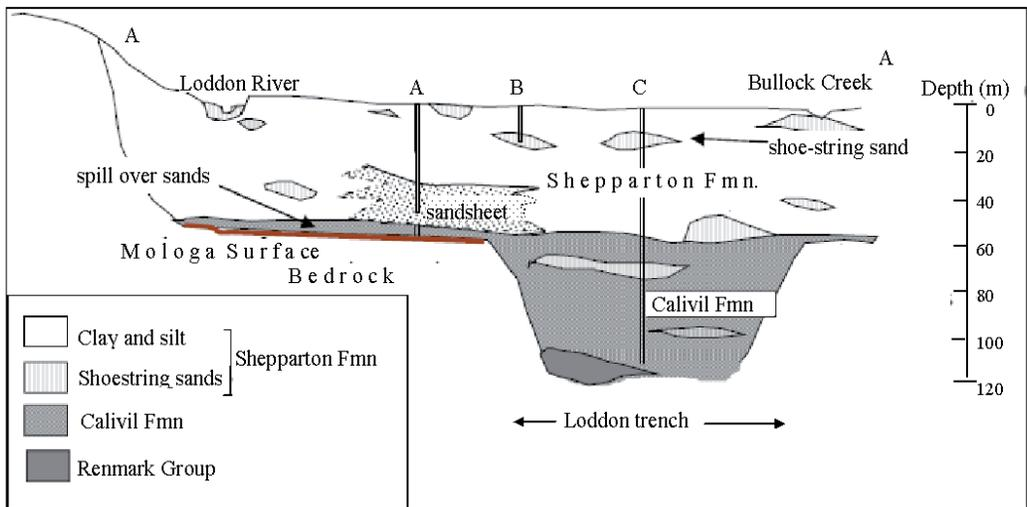
Fig. 10. Diagrammatic figure showing the distribution of sand/aquifer types on the southern Loddon Plain – Section line on Fig. 9.
