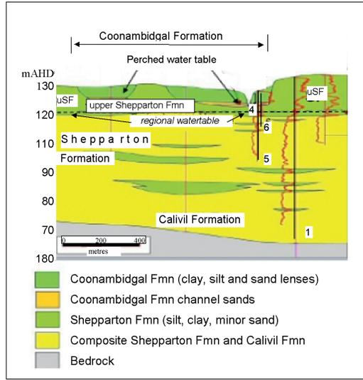
Fig. 25. Geological cross section at Murchison Rd bridge.
