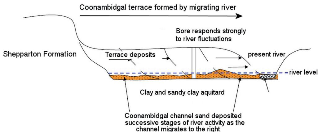
Fig. 17. Relationship between the river, the basal channel sands of the Coonambidgal Formation and the Shepparton Formation at Avonsmore Bridge (diagrammatic).
