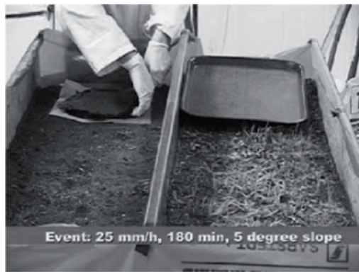
Fig. 2. Testing the effect of vegetation cover on release of Cryptosporidium from artificial cowpats during rainfall events.
