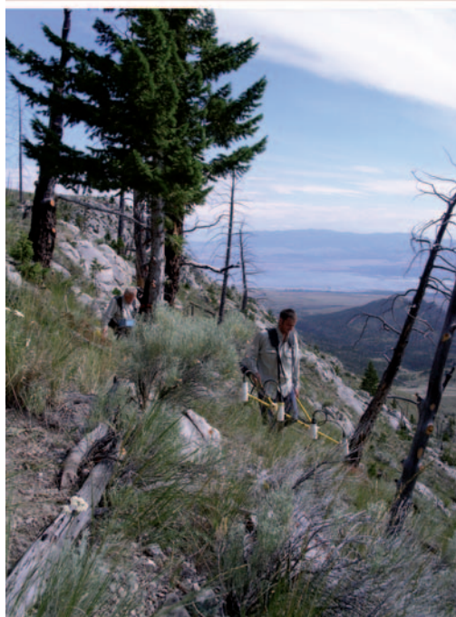
Figure 6. The TM-4 magnetometer with odometer attached. Seen also in quad-sensor application in the search for unexploded ordnance 2000 m above the Missouri valley in Montana.
