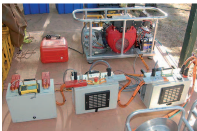
Figure 9. The MPTX-500 transmitter was developed as an EM source capable of delivering up to 350 Amp current through an energising square loop of 110 m x 110 m. When such a loop surrounded a 1 ha search area SAM technology, using a TM-6 magnetometer, was capable of detecting UXO targets down to 20 mm projectile size.
