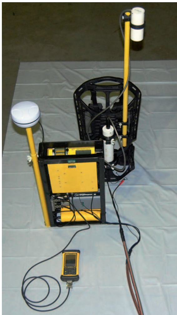
Figure 10. The TM-7 magnetometer system is the current generation. Its performance is similar to that of the TM-6 but advantage has been taken of advanced acquisition electronic components, firmware and processing software.
