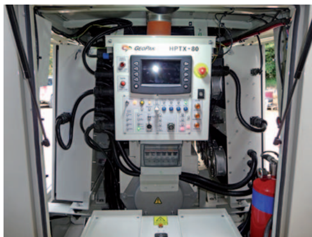
Figure 11. The HPTX-80 transmitter is capable of delivering 80 kW of electrical power to either a galvanic source, where electrodes may be separated by several km, or to an electromagnetic loop of several square km area. With such a transmitter, and the TM-7 magnetometer, very deep electromagnetic exploration can be achieved using SAMSON technology or the survey efficiency of a helicopter-borne platform can be applied to TMI and TFMMR exploration using SAM technology.
