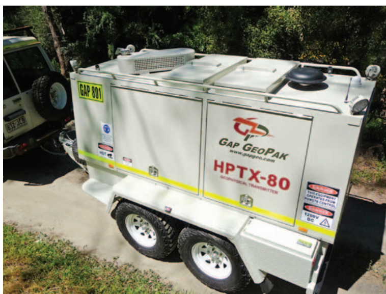
Figure 11. The HPTX-80 transmitter is capable of delivering 80 kW of electrical power to either a galvanic source, where electrodes may be separated by several km, or to an electromagnetic loop of several square km area. With such a transmitter, and the TM-7 magnetometer, very deep electromagnetic exploration can be achieved using SAMSON technology or the survey efficiency of a helicopter-borne platform can be applied to TMI and TFMMR exploration using SAM technology.
