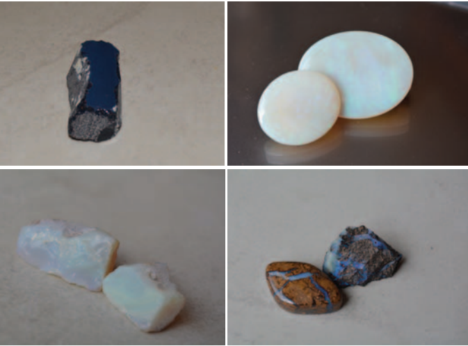
Figure 4. Some of the opaline materials used in the physical property tests prior to shaping for the measurement jigs: top left - Lightning Ridge NSW blue-black common opal, 13.57 g, top right - Coober Pedy SA white opal, 2.95, 5.63 g, bottom left – Coober Pedy SA milky blue common opal, 10.67, 6.50 g, bottom right, – Yowah Qld boulder opal, polished 19.40 g, rough 17.23 g. Photos by Lainie A Kalnins/CC BY-SA 3.0.
