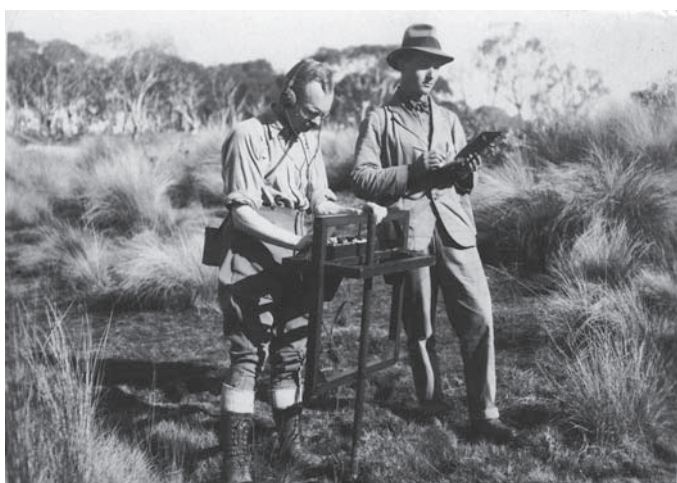
Dr Bieler (on left) using the Bieler-Watson double detecting coil for electromagnetic measurements. Dr Bieler, an expert in electromagnetic methods from McGill University in Canada, joined the IGES as Deputy Director however he died at an early stage in July 1929.
