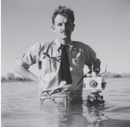
Lew conducting a magnetic survey for AGGSNA in a lake near Wiluna WA, using a Watts Variometer (note the black knitted tie).
