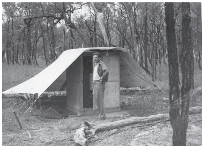
Lew outside a hut used by IGES for gravity gradiometer measurements. This portable kapok lined canvas hut protected the gradiometer from temperature changes and wind.
