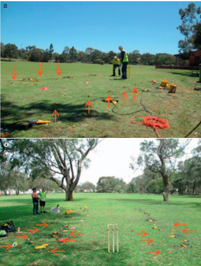
Figure 3. Photos of the (a) initial and (b) improved layouts. The positions of some of the geophones are indicated by red arrows.
