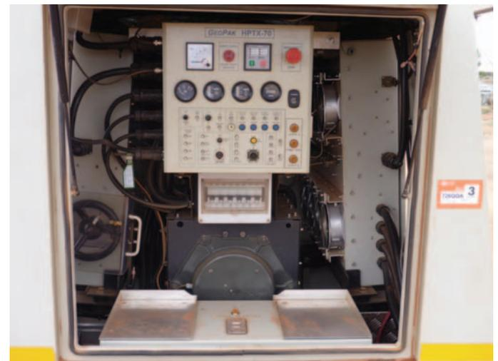
**Fig. 5.** Rear view of the HPTX-70 with the rear door open showing the grey alternator, control module at top and capacitor box at the bottom. The switch module (with voltage selection wheel) is located on the left side. The transmitter module is located on the right.
