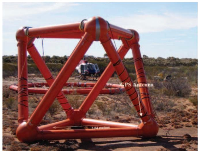
Fig. 3. ZTEM and AirMt base station sensor.
