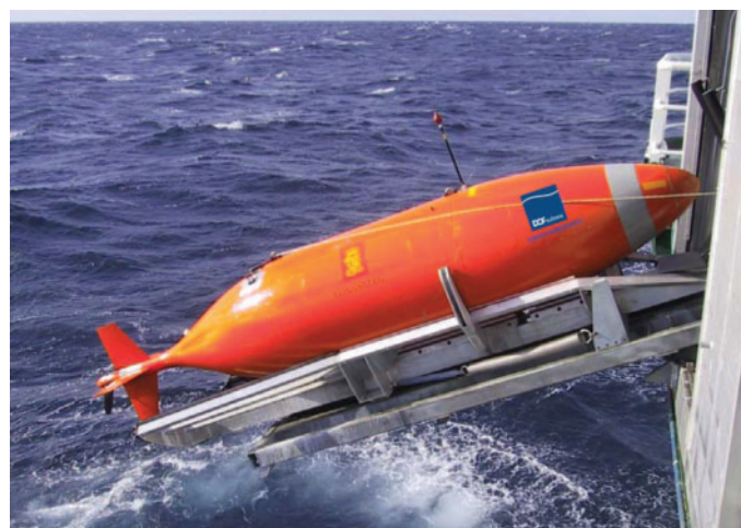
Fig. 2. Hugin autonomous underwater vehicles about to be launched.
