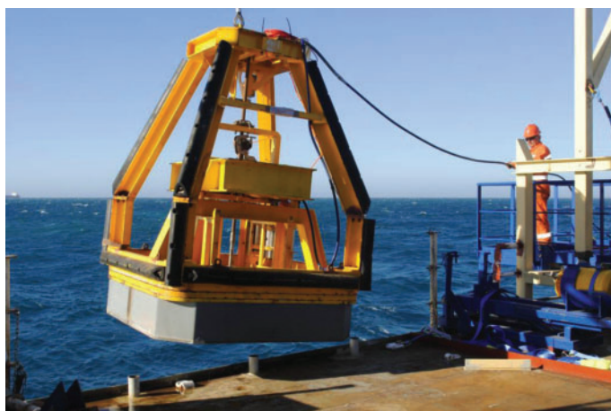
Fig. 4. Cone penetrometer testing being launched off side of the Geobay.
