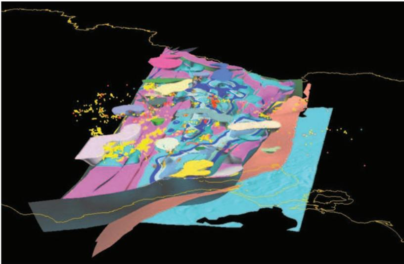
**Fig. 5.** 1:250 000 scale geology model of the Bendigo structural zone. This model shows the basement geology model including all known mineral deposits in the region (red dots = alluvial gold and gold dots = hard rock gold). The view is to the NNW. Image courtesy of Geoscience Victoria.
