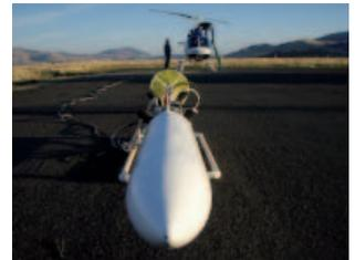
Ultra high resolution magnetics / electromagnetics for UXO and environmental mapping
