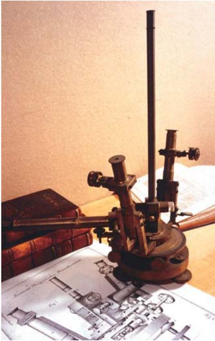
Fig. 4. A surviving Reisetheodolit. Lamont manufactured forty five of these instruments. Image courtesy of Professor Heinrich Soffel, University of Munich.
