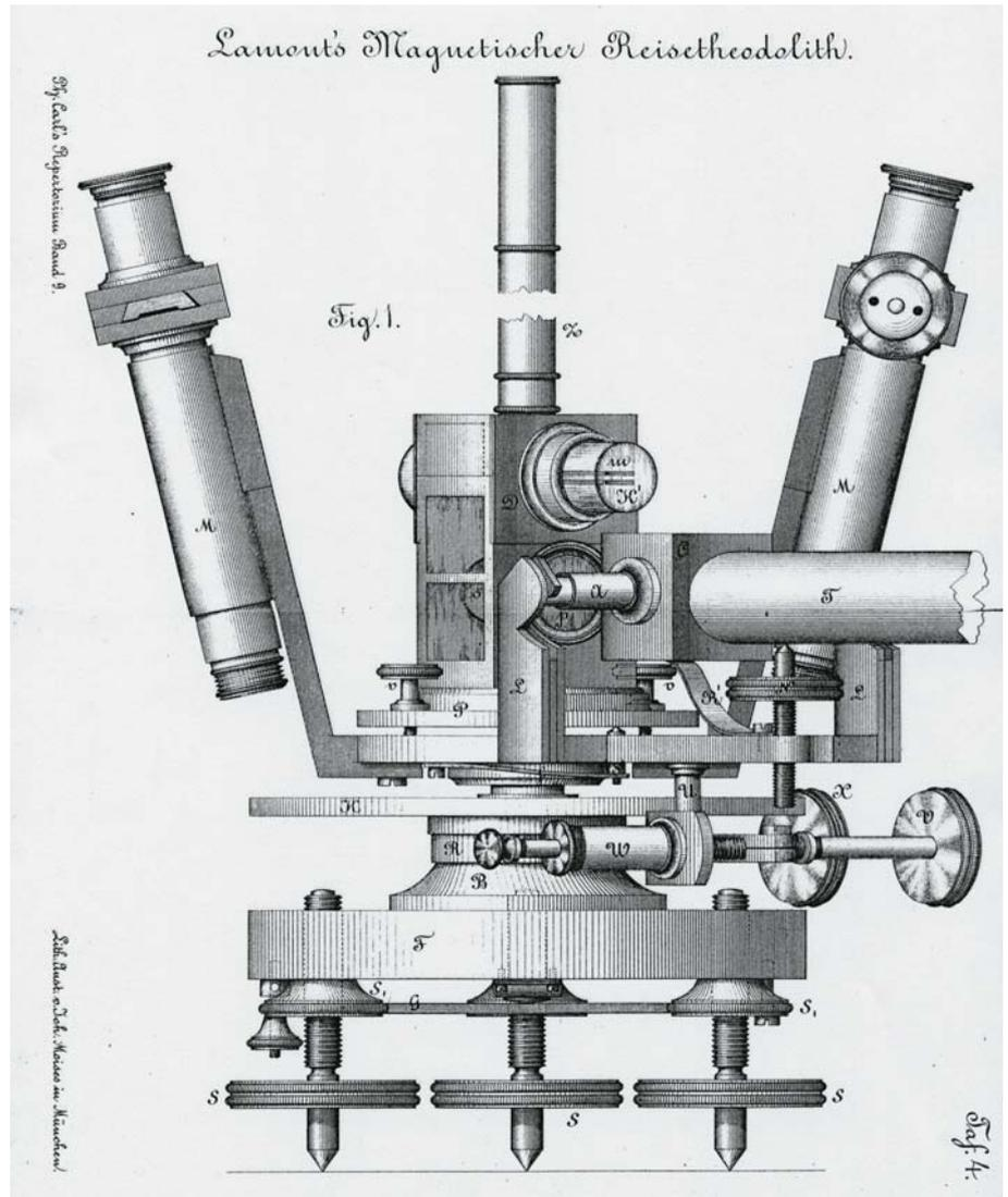
Fig. 5. Lamont's combined declination, inclination and horizontal intensity "Reisetheodolit". Neumayer measured all of his Victorian field measurements using a similar instrument. Image courtesy of Professor Heinrich Soffel, University of Munich.
