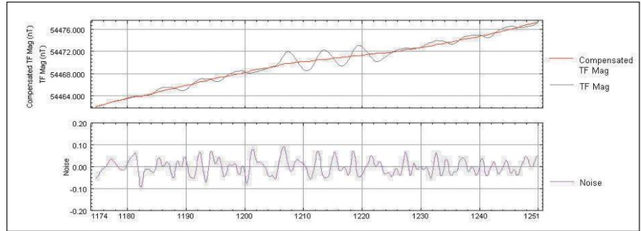
Fig. 5. GeoRanger I.32 nT Figure Of Merit flown at MOA Boardman Oregon in August 2004.
