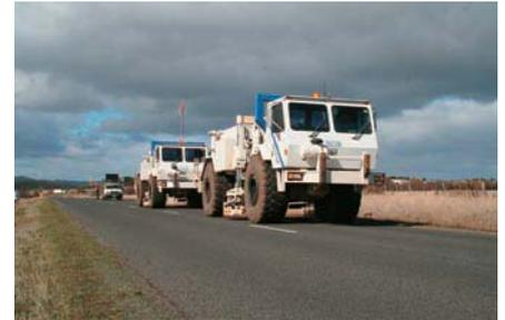
Fig. 4. ANSIR vibrators working hard on the road.
