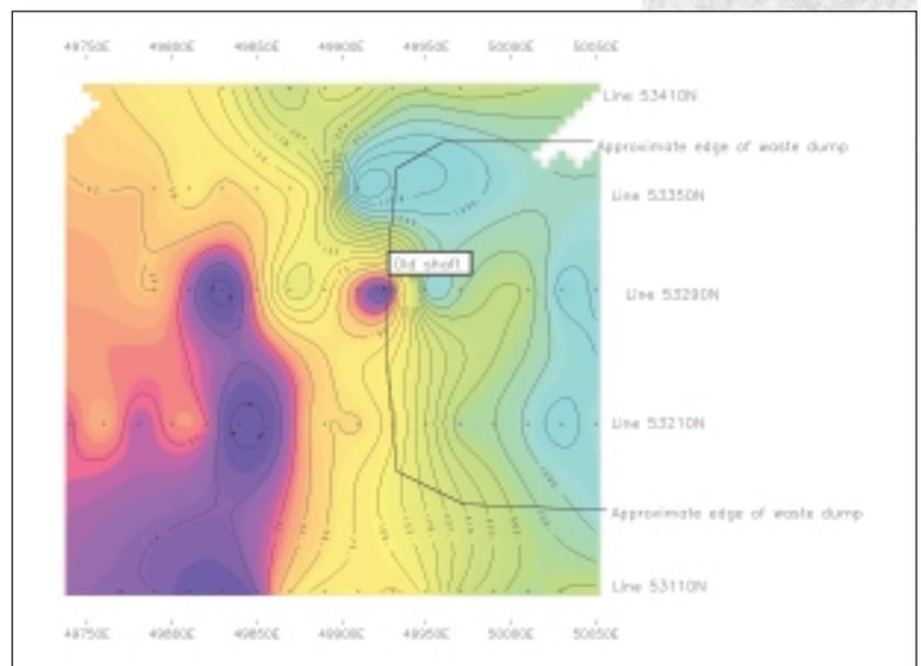
Fig. 10. (Right) Acid Mine Drainage; contoured "depth slice" at 30 m depth created from the one-dimensional inverted sections of all five lines. Note the more conductive zone extending to the west and south of the waste dump - possibly acid-mine runoff.
