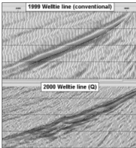
Fig. 5. (Top) Conventional and Q data examples showing the improved resolution in the Q data.
