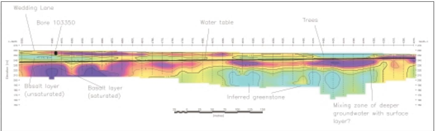
Fig. 7. (Top) Two-dimensional section for the top 100 m of ground along Helen's Road, Willaura Catchment. Resistivities vary from  $> 25 \Omega\cdot\text{m}$  to less than  $< 1 \Omega\cdot\text{m}$ .
