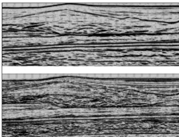
Fig. 6. (Above) Conventional and Q data examples. Data recorded by conventional arrays smear energy across CMPs; improved lateral resolution results from recording single sensors.
