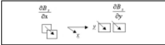
Fig. 2. Arrangement of SQUID sensors for detection of axial and transverse gradients.
