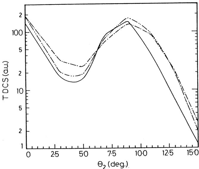
**Fig. 2.** Binary peak values versus peak angles for the triple differential cross section for electron impact energy 250 eV and ejected electron energy 5 eV. Continuous curve, present calculation; dash-dot curve, first Born calculation; and dash-double-dot curve, second Born calculation.
