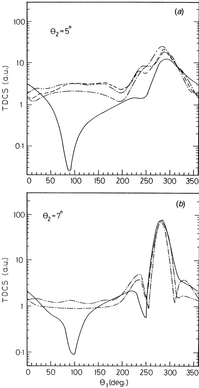
**Fig. 1.** Triple differential cross section versus ejection angle  $\theta_1$  for electron impact energy  $E_i = 250$  eV, ejected electron energy  $E_1 = 5$  eV and for scattering angles  $\theta_2 = 5^\circ$  (1a),  $7^\circ$  (1b),  $9^\circ$  (1c),  $11^\circ$  (1d),  $15^\circ$  (1e) and  $20^\circ$  (1f). Continuous curve, present calculation; dash-dot curve, first Born approximation; dash-double-dot curve, second Born calculation; and dashed curve, BBK theory.
