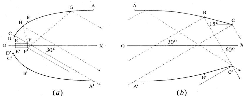
Fig. 2. Details of (a) the collector and (b) the concentrator, illustrating some typical ray paths (see text).
