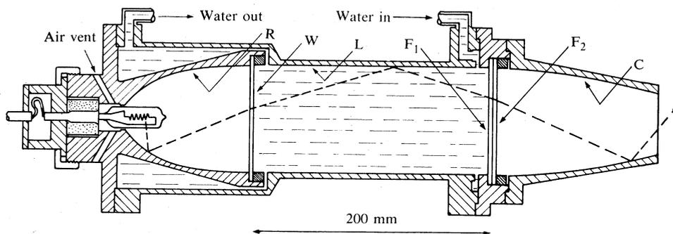
**Fig. 1.** Lamp head and a typical ray path from the filament, reflected once in the collector R, the water filled cylindrical section L, and the concentrator C, emerging through the 53 mm diameter output aperture with a divergence angle from the axis close to the maximum value of  $60^\circ$ . A fused silica window is indicated by W, a coloured glass long-wave pass filter by  $F_1$  and an all dielectric short-wave pass filter by  $F_2$ .
