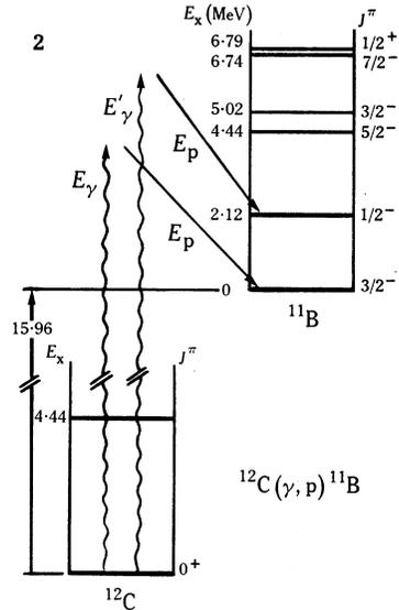
**Fig. 2 (right).** Some energy states involved in photoproton emission from  $^{12}\text{C}$ .
