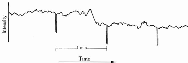
Fig. 1.—Record of immersion of 0316+16 on 1965 February 9 as observed at 2650 MHz. The flux density from this source at this frequency is 4.8 f.u. ( $4.8 \times 10^{-26} \text{ W m}^{-2} \text{ Hz}^{-1}$ ; Shimmins, Clarke, and Ekers 1966).
