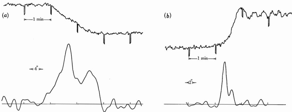
Fig. 3.—Occultation observations and restored distributions for (a) the immersion of 0307+16 on 1965 September 15 and (b) the emergence of 1859-23 on 1964 August 19. The flux densities from the sources at the frequencies of observation are approximately 30 f.u. for 0307+16 at 154 MHz and 10 f.u. for 1859-23 at 410 MHz. The effective restored beamwidths are 4'' arc for (a) and 2'' arc for (b).
