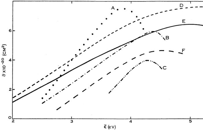
Fig. 4.—Variation of mean cross section  $\bar{\sigma}$  for attachment of electrons with mean energy  $\bar{\epsilon}$ , assuming a Druyvesteyn distribution of velocities.
