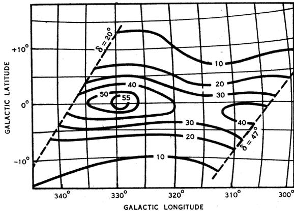
Fig. 1.—Contours of aerial temperature of the region about the galactic centre as seen on the 72-ft reflector at 160 Mc/s (aerial beam width  $6^\circ$  between half-power points). The units are not accurately known owing to uncertainty in the reflection coefficient of the aerial, but the contour interval is approximately  $20^\circ\text{K}$ .
