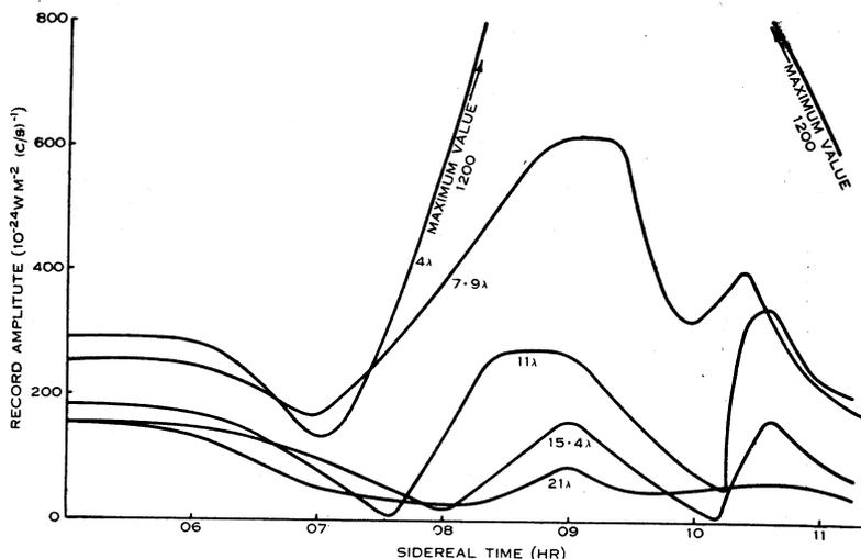
Fig. 7.—Variation in amplitude of the azimuth-interferometer patterns for five aerial spacings. The aerials were directed towards an azimuth of  $40^\circ$ ; the hour angle for a source on the horizon at this azimuth is approximately 08 hr 20 min.
