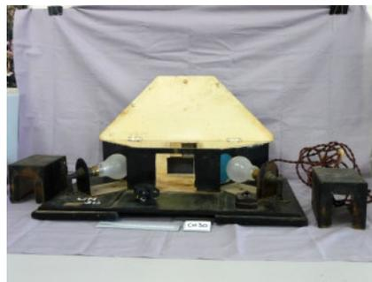
**Figure 1.** The Lovibond Tintometer (partly dismantled) used by Davies in his fish liver oil work (photo: Nola Orr, University of Melbourne Cultural Collections).
