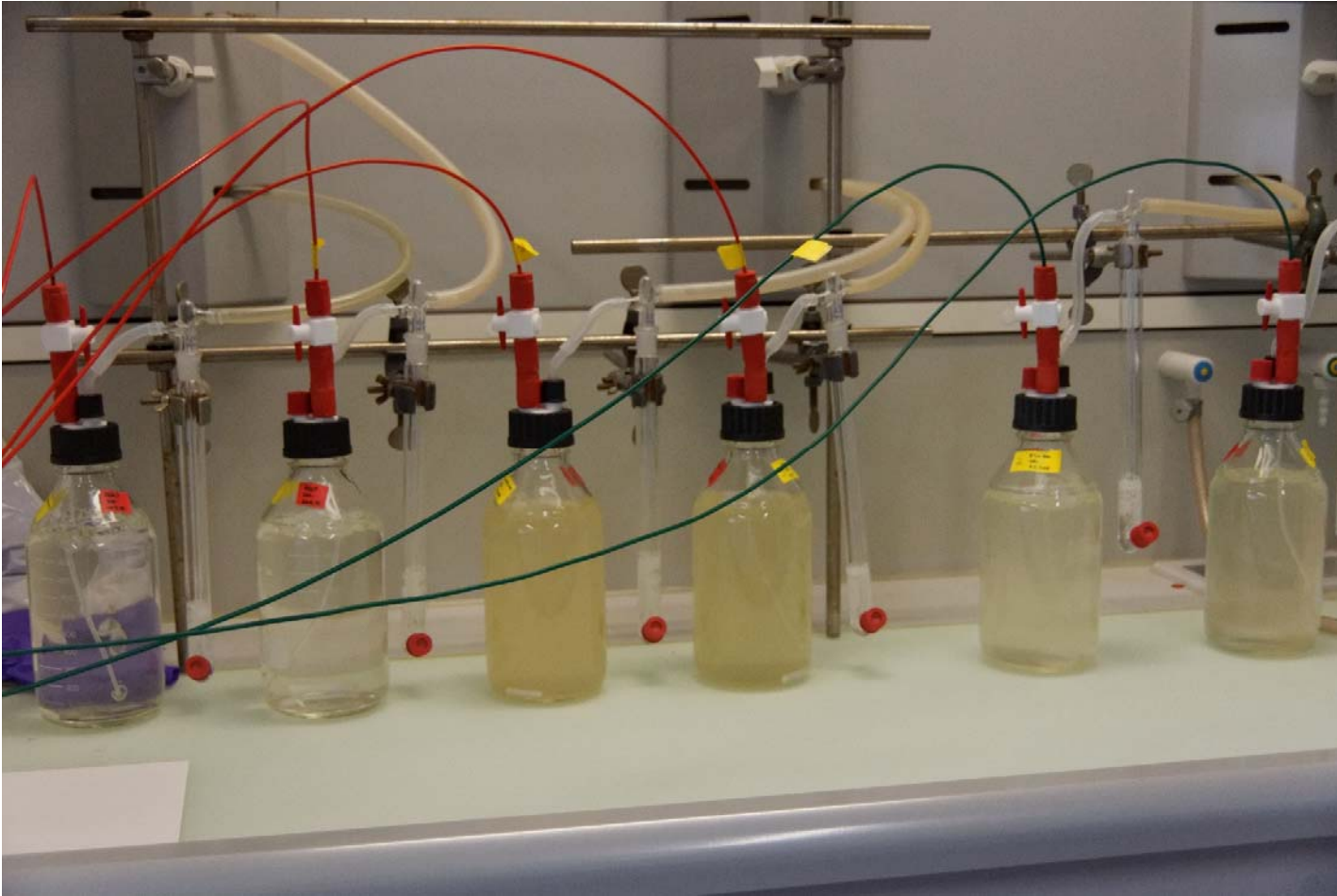
Fig. S3. Acid trapping system used to measure production of volatile S and Se, as described in the materials and methods.
