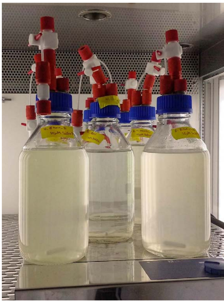
Fig. S2. Batch culture system in Se Volatilisation Experiments. The bottles were gas tight until valves were opened for bubbling at the end of the experiment.
