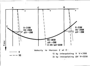
An alternative method is to adopt a standard curve of change in velocity with reflection time, and to smooth the difference between the velocity and the standard velocity, referred to as velocity anomaly. The concept of velocity anomaly can be illustrated with a plot (Figure 1) showing the curves for standard velocity, measured velocity (from analyses) and velocity anomaly plotted against time. This concept may be applied to either moveout velocity or average velocity.
