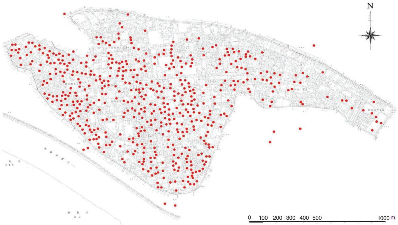
Fig. 8. Distribution of sand boil incidents in the Hinode area (from a report by Itako city). Red dots show the locations of confirmed sand boils. Modified from a figure in a publication by Itako City (2014).
