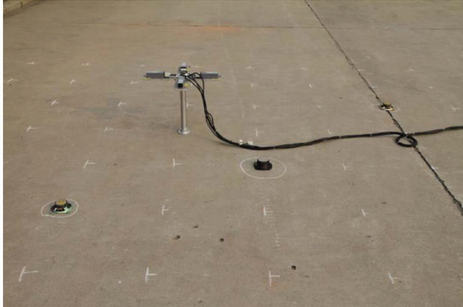
Fig. 6. Experimental system with magnetic gradient tensor system and three magnets.
