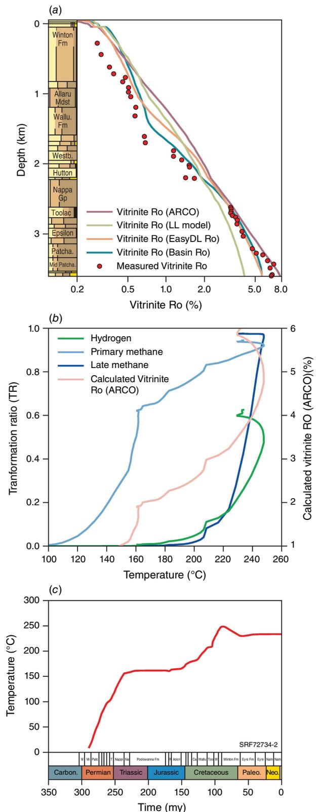
**Fig. 2.** For Burley 2 well (a) modelled and measured vitrinite reflectance (Vitrinite Ro) versus depth, (b) transformation ratio for primary methane, late methane and free H<sub>2</sub>, and modelled vitrinite reflectance versus modelled temperature and (c) modelled temperature history versus age.
