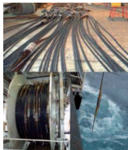
Fig. 6. Optical seabed array being prepared in warehouse, on deployment reel and during deployed.
