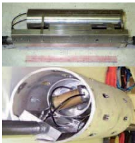
Fig. 5. Sensor pad assembly, side view of geophone housing on sensor pad base, end-on photo with protective housing shows hydrophone mounted in pad.
